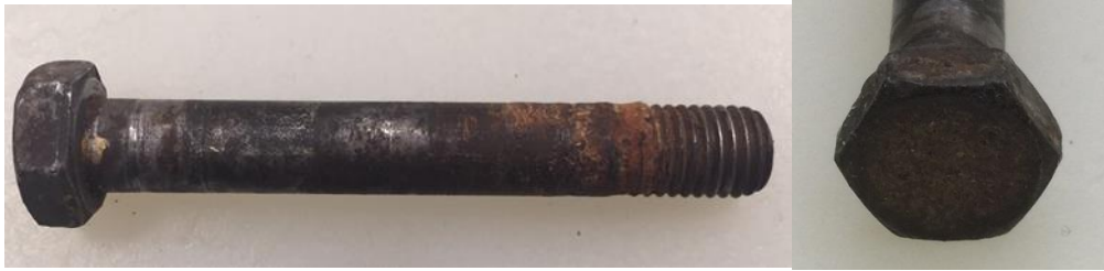
Fig 6. The corroded bolt (Part No. FBA5-21A) that held the partially failed side cable to the control frame.
