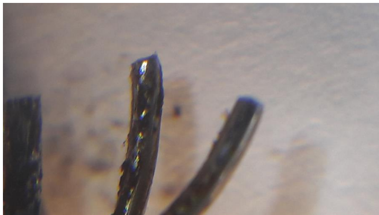
Fig 5. Failed cable strands showing wear grooves and corrosion pits.
