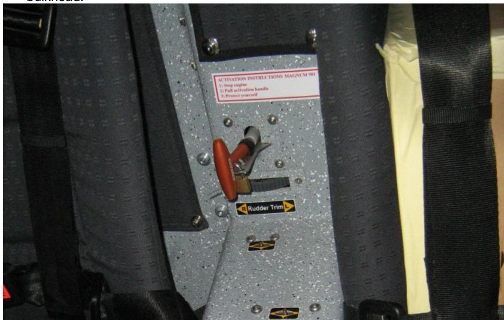
Handle mounting (Junkers shown, BRS is similar)
