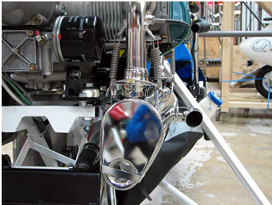
Fig 4 Exhaust springs and backup cable
