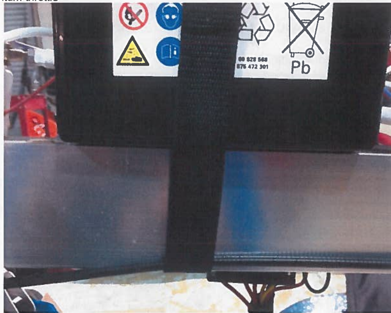
Fig 2 Secure the throttle cable under the battery strap as shown.
