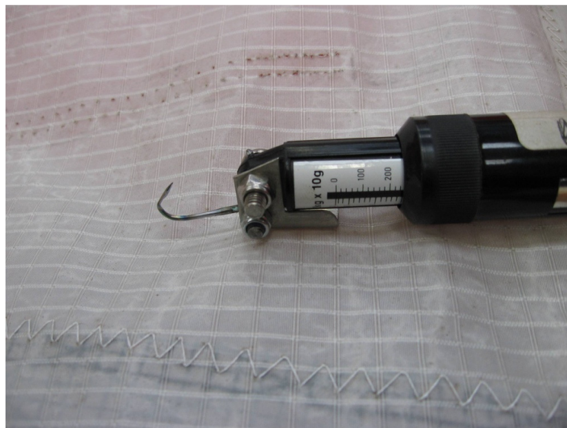
Fig. 4 Bettometer test – HTP square material, note the rip-stop weave. The fine fibres within each square are tested. Test load must not rip the small square between each ripstop cord
