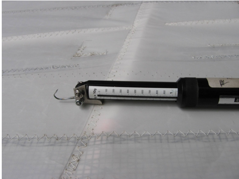
Fig 3. Bettometer test, plain sailcloth
