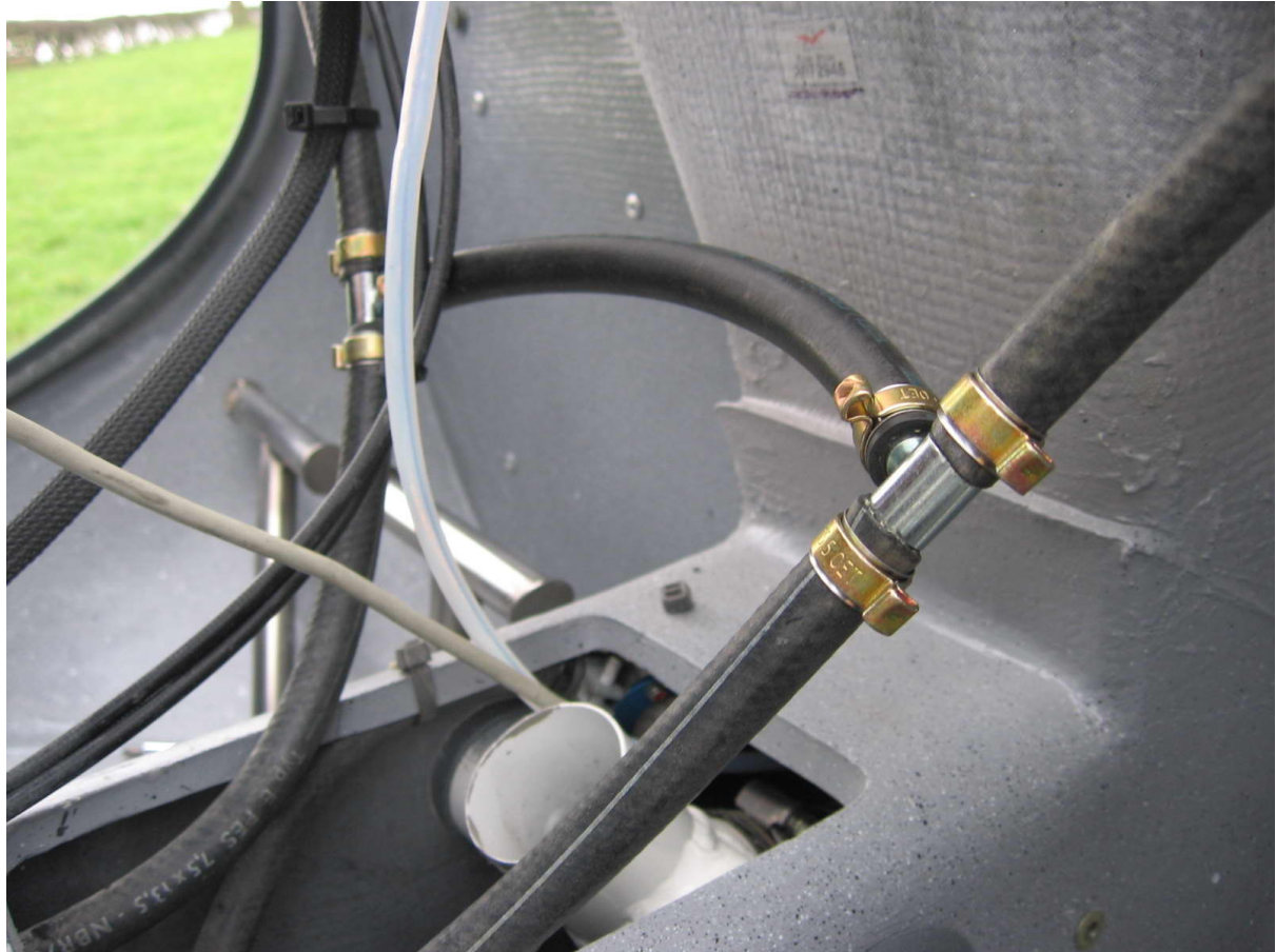
Fig 1 Tee pieces installed approximately 100mm above the top of the tunnel.
