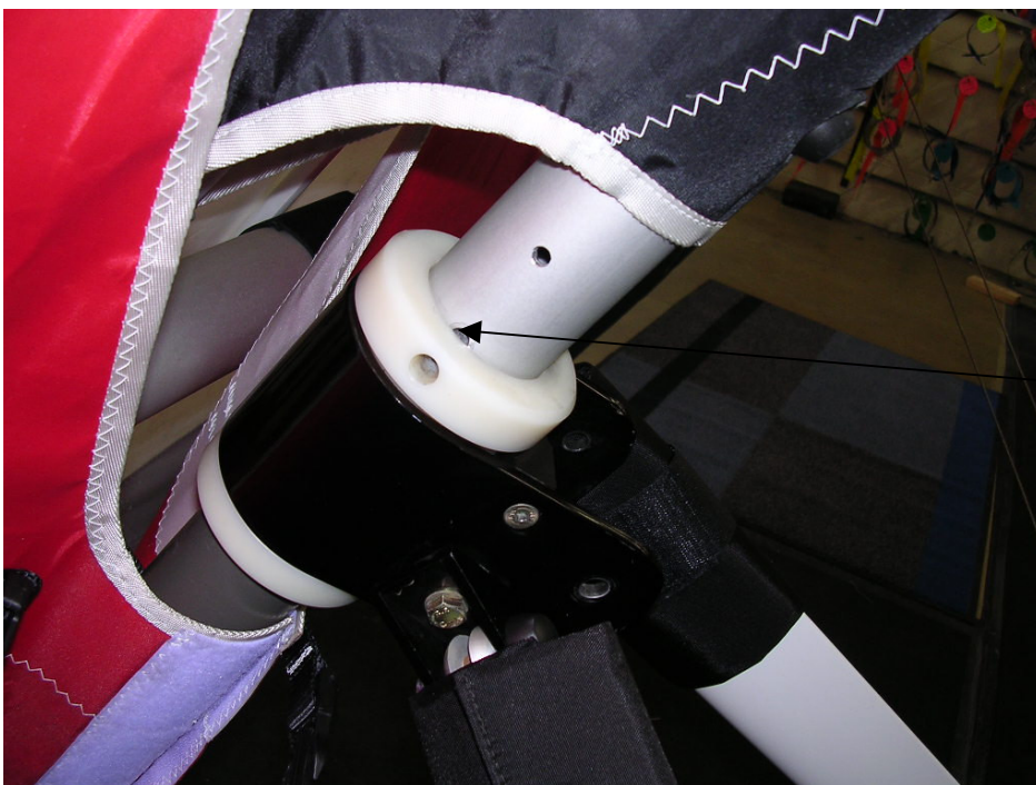
Figure 2 Photo Of Wing showing roll bracket bearing slid fully forwards.
