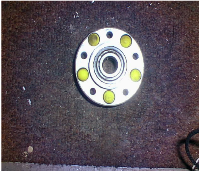
Foam plugs inserted in lightening holes.
