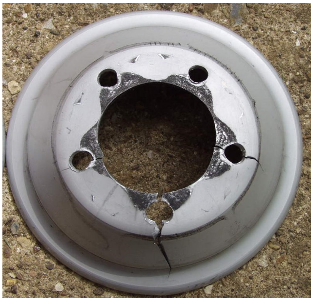
Failed hub showing extensive fretting due to loose bolts before failure.
