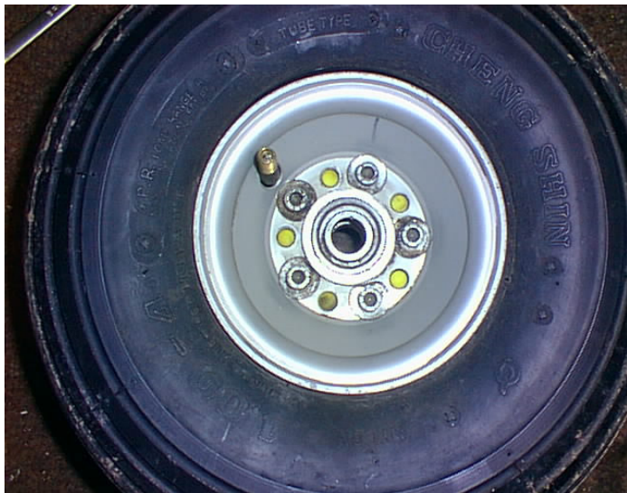
Hub assembled correctly showing foam plugged lightening holes.
