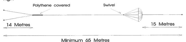
A short length of polythene covered cord between the bridle and the main line keeps the bridle from twisting up on landing. A parachute is provided in the main line approximately 15 metres from the glider. It forms part of the tow line itself and therefore closes under towing tension and opens automatically once the glider has released. The main line cord is made from stiff material with very good stretch properties.
